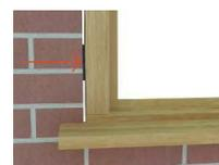
Cill and head packings should be a maximum of 150mm from each jamb and beneath each mullion. It is very important when fitting to ensure the frame doesn't become distorted as this can prevent movement of sashes, be especially careful for this problem when installing sliding sash windows.
